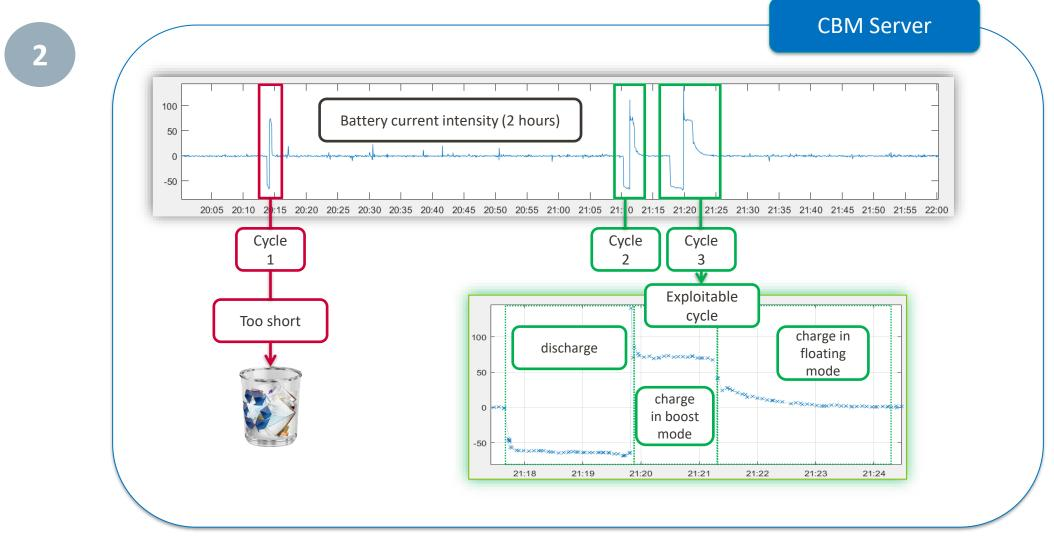
DATA PROCESSING : HEALTH INDICATOR AGGREGATION INTO INDICATOR VECTORS
